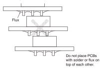
• When performing soldering with a dip soldering bath, ensure that the flux does not reach a higher level than the PCB.
