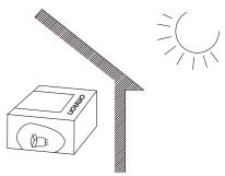
If the Switch is stored in a location where it will be exposed to direct light, colored resin in the colored plate may fade. Therefore, do not store the Switch in locations where it will be exposed to direct light.
