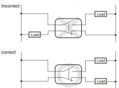
Connect the load to the same polarity.
