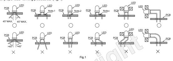
Correct mounting method "X" Incorrect mounting method
