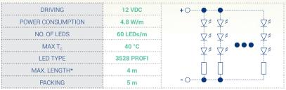
$^{\star}\delta$  20 = 80 sections (1 section = 50 mm) is the length of LED ribbon from the connection, at which lumen depreciation reaches 20%.
