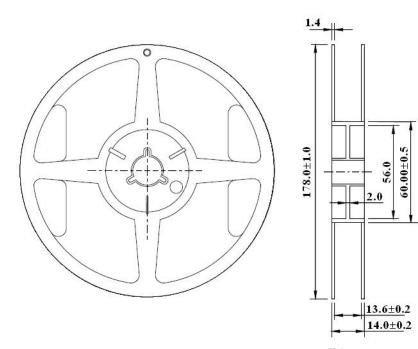
Unit: mm Tolerance: ±0.25mm
