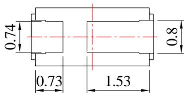
**Recommended Soldering Pad Dimensions**
