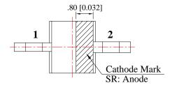
Unit: mm Tolerance:  $\pm 0.10$  mm
