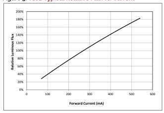
Figure 4: V10C Typical Relative Flux vs. Current
