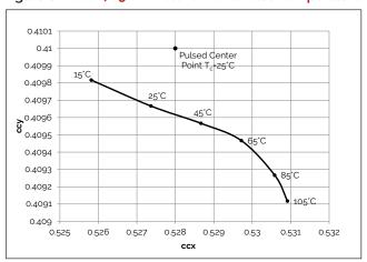
Figure 10: 2700K, 97 CRI Color Shift vs. Case Temperature<sup>1</sup>
