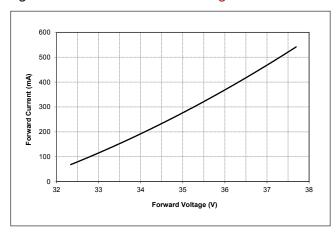
Figure 2: V10C Drive Current vs. Voltage
