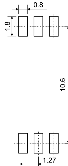
Fig. 15.2 Lead Forming Option (LF4)
