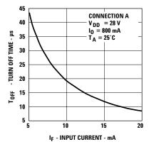
Figure 15. Typical Turn Off Time vs. Input Current.
