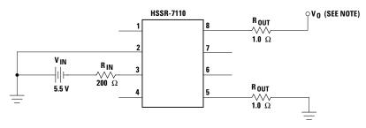
NOTE: IN ORDER TO DETERMINE V  $_{\text{OUT}}$  Correctly, the case to ambient thermal impedance must be measured for the burn-in boards to be used. Then, knowing  $\,\theta_{\text{CA}}$ , determine the correct output current per figures 2 and 4 to insure that the device meets the defailing requirements as shown.
