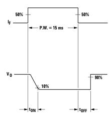
Figure 10. Switching Test Circuit for  $t_{\text{ON}}$ ,  $t_{\text{OFF}}$ .
