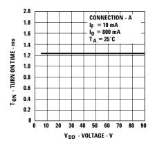
Figure 13. Typical Turn On Time vs. Voltage.
