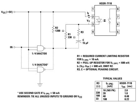
Figure 1. Recommended Input Circuit.
