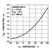
Figure 11. Typical Turn On Time vs. Temperature.
