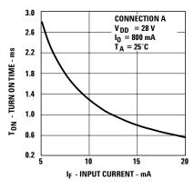
Figure 12. Typical Turn On Time vs. Input Current.
