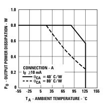
Figure 4. Output Power Rating vs. Ambient Temperature.
