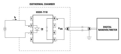
Figure 19. Voltage Offset Test Setup.
