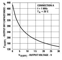
Figure 16. Typical Output Off Capacitance vs. Output Voltage.
