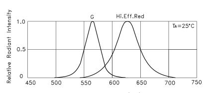
wavelength  $\times$  (nm) RELATIVE INTENSITY Vs. WAVELENGTH
