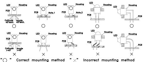
During soldering, component covers and holders should leave clearance to avoid placing damaging stress on the LED during soldering.
