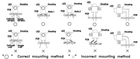
2. During soldering, component covers and holders should leave clearance to avoid placing damaging stress on the LED during soldering.
