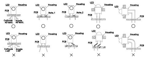
"Correct mounting method "X" Incorrect mounting method
