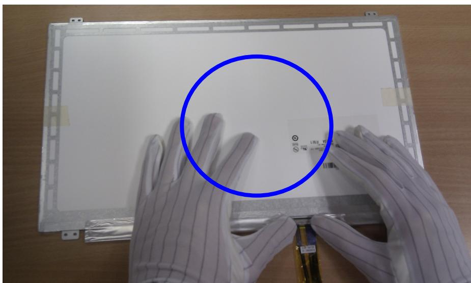
Insert the connector by pushing right and left edge.
