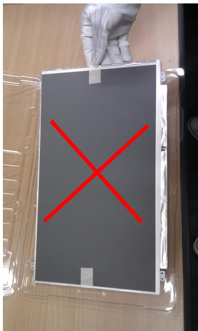
Do not lift and hold the panel with single hand at right or left side from tray.
