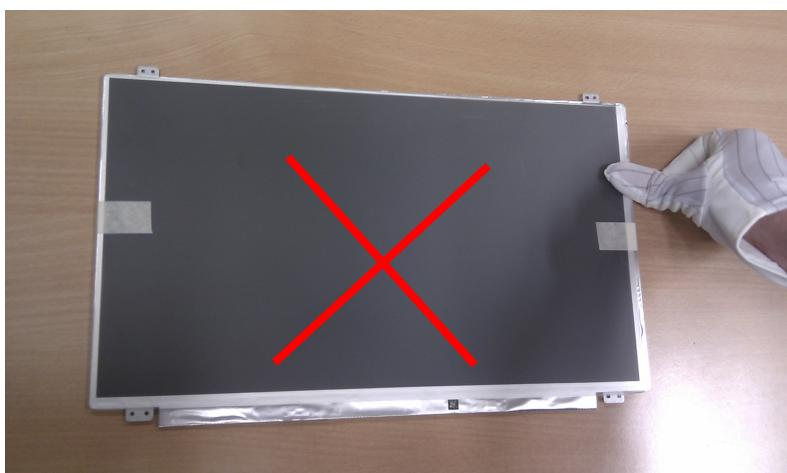
Do not press edge of panel to avoid glass broken.
