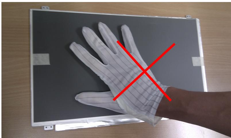
Do not press the surface of the panel to avoid the glass broken or polarizer scratch.
