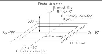
Fig. 9.2. Optical measurement system setup
