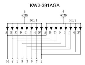
Internal Circuit Diagram (Common Cathode)
