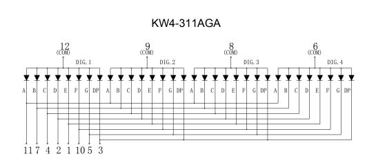
Internal Circuit Diagram (Common Anode)
