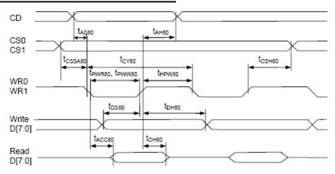
Parallel Bus Timing Characteristics (for 8080 MCU)
