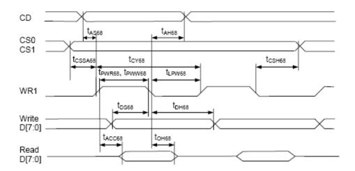
Parallel Bus Timing Characteristics (for 6800 MCU)
