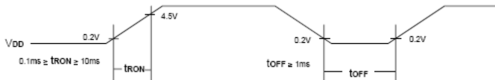
Figure 3. tOFF stipulates the time of power OFF for instantaneous Power supply to or when power supply repeats ON and OFF
