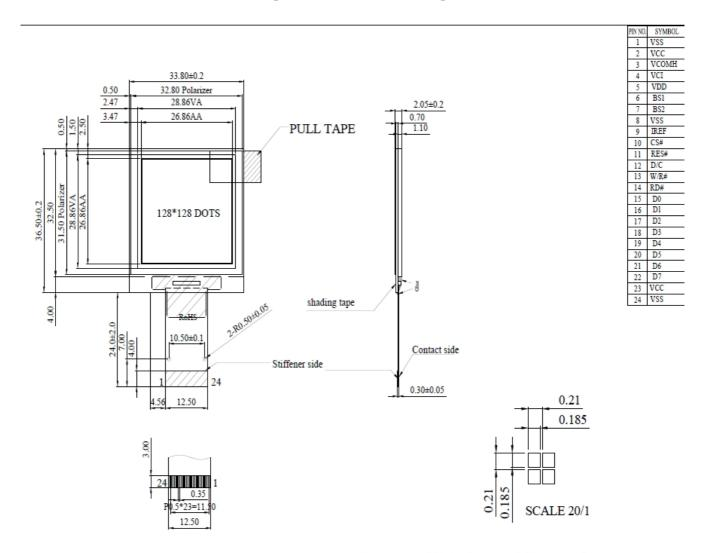
The non-specified tolerance of dimension is  $\pm 0.3$ mm.
