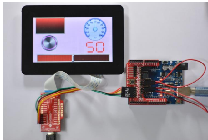
Figure 3. gen4 display (gen4-uLCD-43DCT-CLB), connected to the 4D-UPA using 30-way FFC cable, and a 5-way cable connecting to the Arduino Adaptor Shield, on top on an Arduino.
