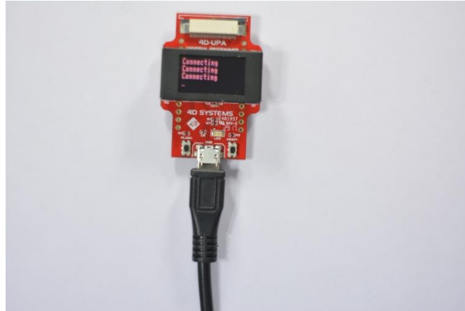
Figure 1. Connection of an IoD-09TH Display module to 4D-UPA with a \mu USB Cable.
