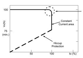
Typical LED power supply I-V curve
