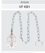
Accessories See page 5/1 All measures in the drawings are in mm page 4/79 Actuator entry locking device Padlockable device to lock the actuator entry in order to prevent from the accidental closing of the door behind operators while they are inside the machine. To be used only with FD, FL, FC and FS series with metal heads.
