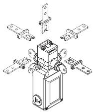
The head can be quickly rotated on each of the 4 sides of the switch by unfastening the two fixing screws. The mechanical lock release device can be rotated in 90° steps as well. This enables the switch to assume 32 different configurations.
