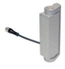
This version with cable and M12 connector from back is the best combination between aesthetics and connection ease. When machineries have to be assembled by the final customer, this solution allows to hide the wiring and at the same time to easily connect or disconnect it from inside the machinery.
