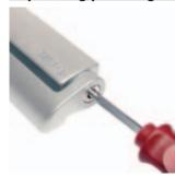
The switches operating point can be regulated through a simple Phillips screwdriver. The operating point regulation allows the setting possibility (up to 4°) for large guards. After the setting, it's always necessary to close the hole through the suitable supplied safety seal plug.
