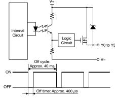
The safety outputs of the SafetyOne are solid state outputs. When the output is on, off-check signals are generated at regular intervals. The operating characteristics of the safety output change depending on the selected logic. For details, see user's manual "Chapter 5 Logic." The basic specifications remain the same.
