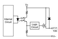
The selected operating characteristics of solenoid/ lamp output change depending on the selected logic. For details, see user's manual "Chapter 5 Logic." The basic specifications remain the same. Do not use solenoid/ lamp output as a safety output, otherwise the sys-tem's safety cannot be assured when the SafetyOne or safety components fail.
