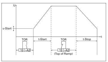
Figure 5. Start and stop ramp functions
