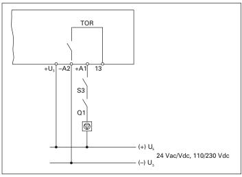
Figure 4. Direct start control wiring with soft stop
