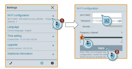
Note that the new Wi-Fi configuration can be effective only after SINAMICS V20 Smart Access restarts.
