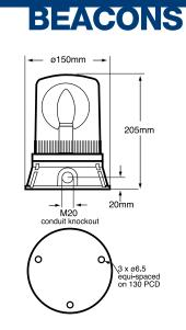
The R401/400 Din Base Series uses a parabolic reflector which, driven by an electric motor, revolves around a continuously illuminated lamp on the vertical axis of the beacon creating a powerful beam of light travelling through 360
