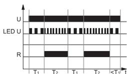
When the supply voltage U is applied, the set interval T1 begins (green LED flashes slowly). After the interval T1 has expired, the output relay R switches into on-position (yellow LED illuminated) and the set interval T2 begins (green LED flashes fast). After the interval T2 has expired, the output relay switches into off-position (yellow LED not illuminated). The output relay is triggered at the ratio of T1:T2 until the supply voltage is interrupted.
