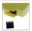
Redundant Dual Power Input: A second power supply can be fitted as a back-up to prevent down time should one power source fail.
