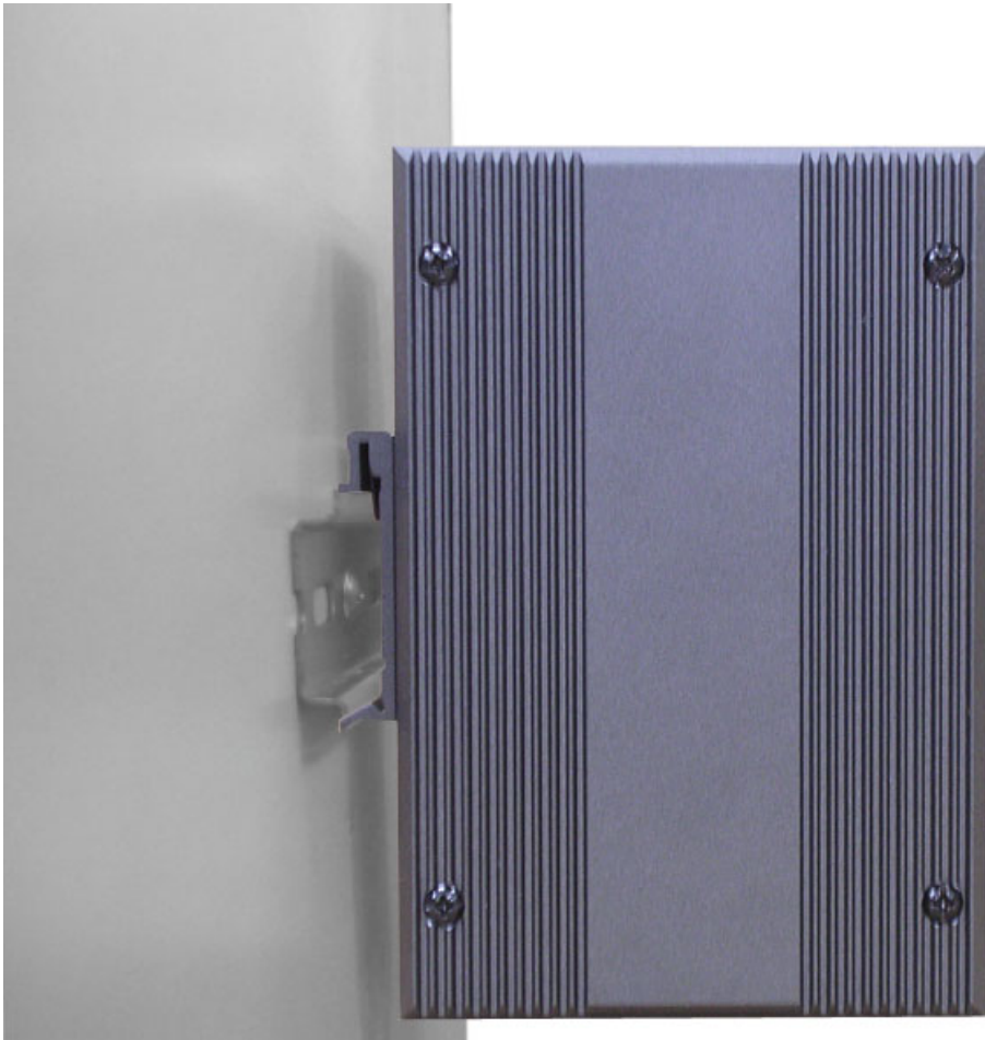
Figure 2.7: Installation to DIN-rail Step 2
