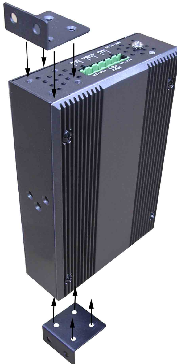
Figure 2.5: Combine the Metal Mounting Kit
