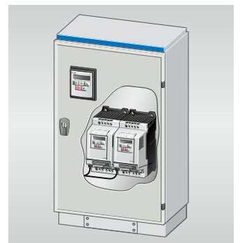
Up to 63 devices can be accessed through a keypad mounted in the control panel.
