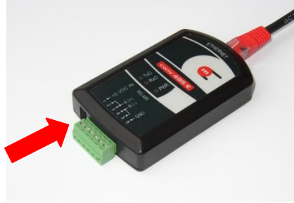
Figure 2.1 Termination switch location
