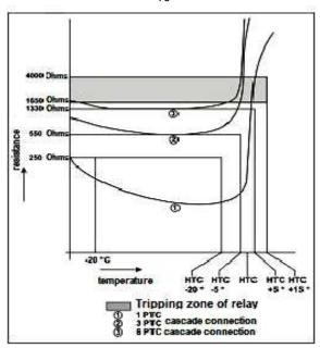
Picture 3 – Resistance-Temperature diagram of PTC sensors
