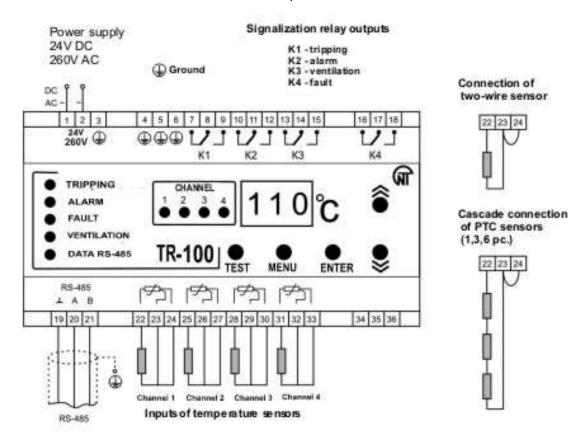
Picture 2 – Electrical connections of TR-100
