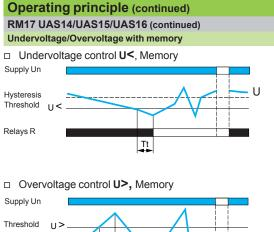
If "Memory" mode is selected, the relay opens when crossing of the threshold is detected and then stays in that position. The power needs to be switched off to reset the product.
