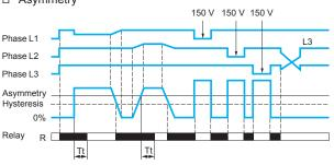
□ Control of overvoltage and undervoltage in window mode <U<
