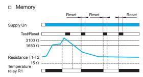
Relay version RM35TM250MW has a "Test/Reset" button which can be used to check that the temperature control function is working correctly and to reset this function after locking in "memory" mode.
