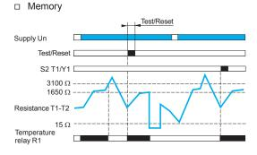
Relay RM35TM250MW has a selector switch which allows the temperature control operating mode to be configured with or without memory.
