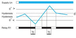
After a delay on pick-up after energization, and for as long as the temperature monitored by the PT100 probe remains between the two threshold settings on the front panel, the temperature relay R1 is closed.
