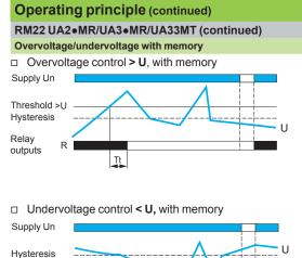
If "Memory" mode is selected, the relay opens when crossing of the threshold is detected and then stays in that position. The power has to be switched off to reset the product.
