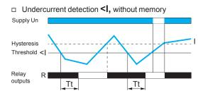
If the controlled current falls below the threshold setting for a time greater than that set on the front panel (0.1...30 s), the output relay opens and the R LED goes off. During the time delay, this LED flashes.
