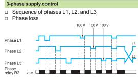
■ As soon as phase sequence (L1, L2, and L3) and phase presence are considered to be correct, the output relay contact closes and LED R2 is lit.
