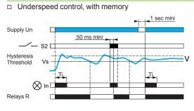
When relay RM35S has been configured in "memory" mode, if underspeed is detected, the output relay stays in the "open" state, irrespective of any further changes in the process speed.
