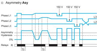
Tt: time delay after crossing of the threshold (adjustable on front panel)
