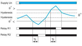
After a delay on pick-up after energization, and for as long as the temperature monitored by the PT100 probe remains between the two threshold settings on the front panel, the output relays are closed and their yellow LEDs are on.
