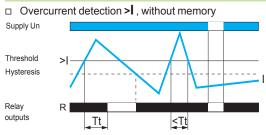
If the controlled current exceeds the threshold setting for a time greater than that set on the front panel (0.1...30 s), the output relay opens and the R LED goes off. During the time delay, this LED flashes.
