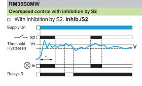
On energization, in order to allow the process being monitored to reach its nominal operating speed, relay RM35S is inhibited for a time delay adjustable from 0.6...60 s. This time delay can be modified (shortened or lengthened) during inhibition. Relay RM35S can also be inhibited by closing of contact S2: on starting, for example, if the process run-up to speed time is greater than 60 s, or at any time during operation.
