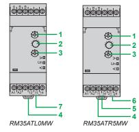
Yellow LED: indicates relay output status (high temperature threshold)
