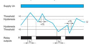
These relays operate in window mode where they check that the controlled current stays between a minimum and a maximum threshold.
