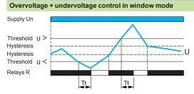
These relays operate in window mode where they check that the controlled voltage stays between a minimum threshold and a maximum threshold.
