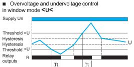
These relays operate in window mode where they check that the controlled voltage stays between a minimum and a maximum threshold.
