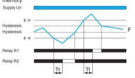
■ If the frequency of the voltage controlled exceeds the over-frequency threshold setting for a time greater than that set on the front panel (0.1...10 s), the corresponding output relay opens and its LED goes off. During the time delay, this
