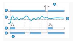
After the end of the inhibit delay on starting, "Ti", as soon as the measured speed rises above the threshold value, the output relay changes state, from operating point to rest position ("alarm" operational state. 11-14 open and 11-12 closed).
