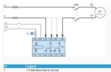
1 A fast-blow fuse or cut-out
