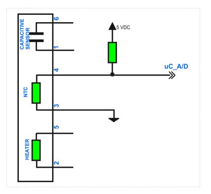
To drive the HEADER measure you can use the following schematics:
