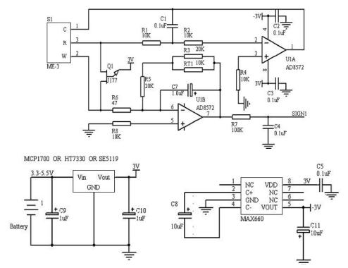
Fig2: ME4-H<sub>2</sub>S test circuit
